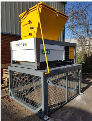
Achieving throughputs of up to 500kg, the flexible RS40 is also capable of shredding wooden pallets and crates that can similarly be volume-reduced to magnify the fiscal benefits of the
