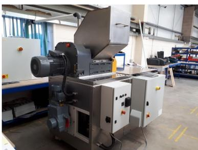
The process sees Advetec's bespoke blend of natural bacteria and stimulants digest the organic content and produce an exothermic reaction which in turn creates a self-sustaining biomass. With each solution tailored to the client's specific requirements, the Advetec XO series can process anything from 500kg to 10,000 kg per day with output material which is dry and has a
