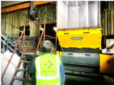
Bespoke plastic recycling company, Meplas, has invested in an LRK1400 shredder from UNTHA UK, to process the 600-tonnes-per-month of hard and soft plastics it receives from the UK's post-industrial manufacturing outlets, at its facility in East Yorkshire.
